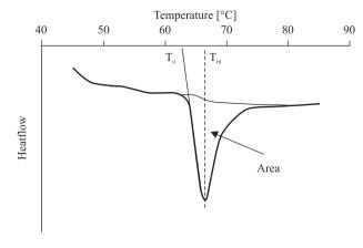
**Figure 1.** A typical DSC thermogram for a peritoneal sample. The curve represents a transition from a native to denaturated state of the sample.  $T_o$  — initial temperature of the transition,  $T_m$  (peak temperature) — temperature of denaturation, the area of the peak is equal to the energy absorbed by the sample during transition
